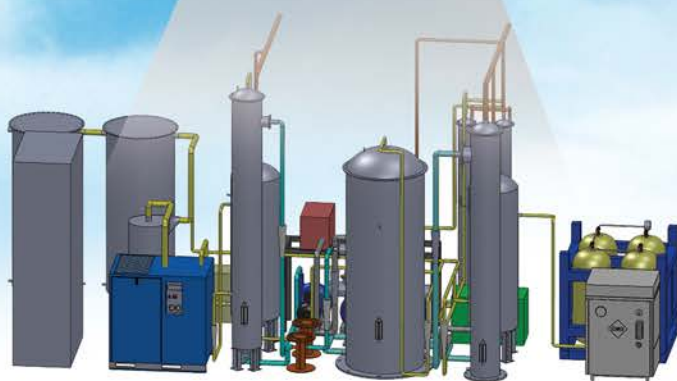
CMU-CBG system (Water Scrubbing Process)
